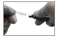
**CAUTION:** When inserting a blade, the blade hole must be seated over the indexing pin. If it is not, the head will be damaged when the locking lever is closed. **DO NOT** force the locking lever if excessive resistance is felt.
