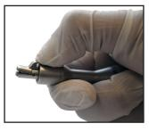
3. Insert the blade between the floating jaw and the indexing pin, making sure to fit the hole in the blade over the indexing pin.
