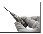
WARNING: Collet must be in full position to prevent overheating of the instrument.WARNING: DO NOT run the instrument without a bur or drill, or the instrument will overheat.
